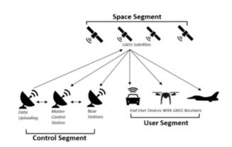
SDR can enable the functionality of both the control, and the user segments, as seen above in global navigation satellite systems. Per Vices SDRs are compatible with all the major GNSS currently used, including GPS (USA), Galileo (EU), GLONASS (Russia) and BeiDou (China).
