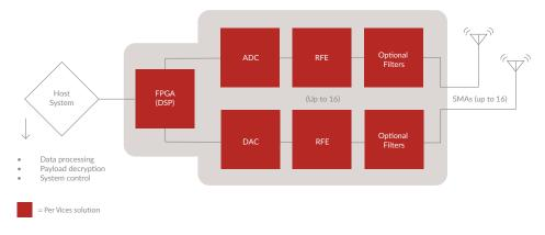
In the SDR's receive chain (left), the incoming signal is fed through a lownoise amplifier, followed by a series of filters and mixers before being digitized for further processing. Higher quality radios have higher quality RF front-ends and are better at locking signals, even when they are weak. Having a nice clean signal digitized quickly means that more of your processing can be done in software.
